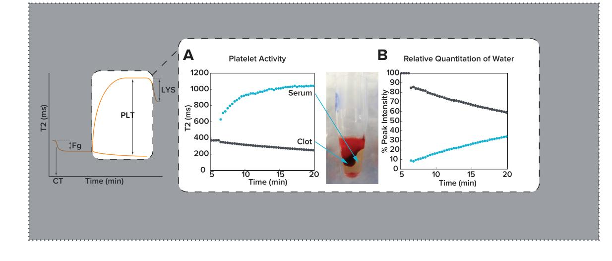
Figure 7. Example of T2MR data. A whole blood sample was activated with an ellagic acid reagent. A) Activation of platelet results in distinct T2 values associated with the fibrin clot (gray) and
