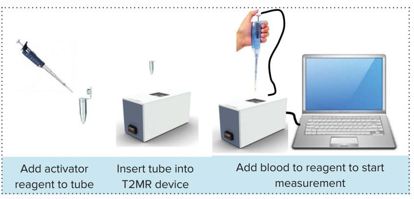
Figure 2: Schematic of procedure to obtain multiplexed hemostasis T2MR measurements.
