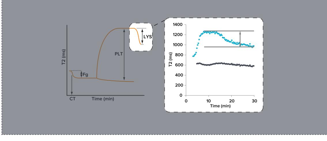
Figure 9. Example data from a whole blood sample that was spiked with tPA. After the initial formation of the contracted clot the T2 values associated with the serum start to decrease as the contracted clot is broken down and RBCs are released into the serum.
