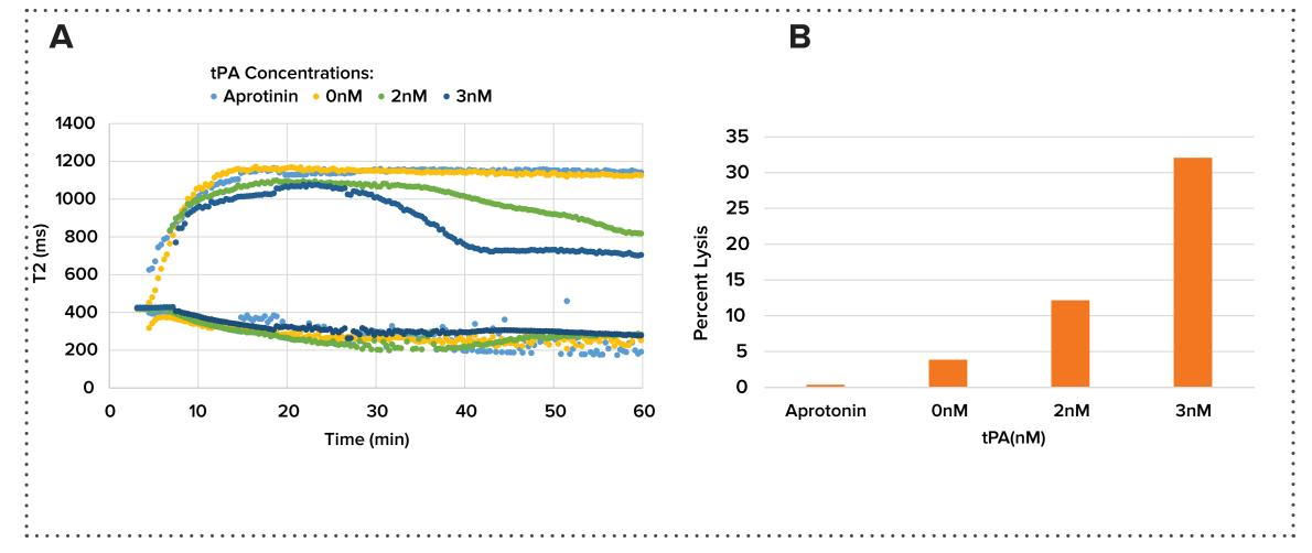
Figure 10. Fibrinolysis was induced in citrated whole blood samples by adding tPA to samples. A) Example T2MR data of blood samples containing 0 – 3nM tPA or the fibrinolysis inhibitor Aprotinin. B) Percent lysis was determined by calculating the percent change in T2 values of the serum peak at 45
